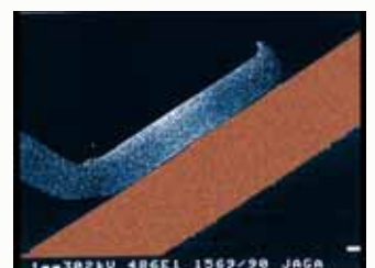
Microscopic view of the aluminium fins attached to the copper tube
